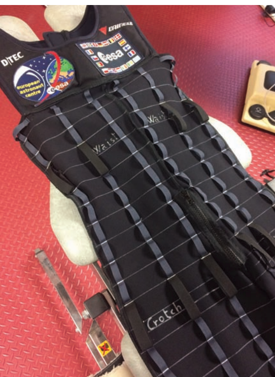
Gravity Loading Countermeasure SkinSuit
